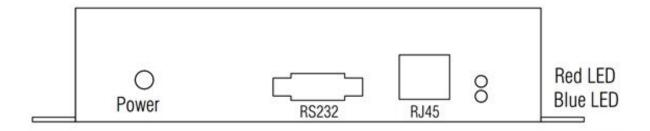
Red: ON for normal work and BLINKING for abnormal warning such as antenna broken.
