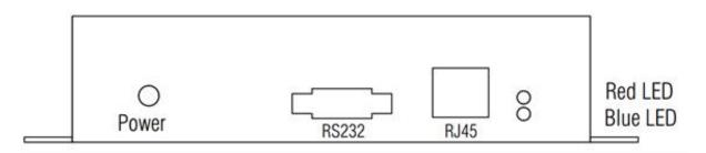
Red: ON for normal work and BLINKING for abnormal warning such as antenna broken. Blue: ON for command executing and OFF for idle state.
