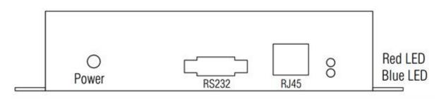
Red: ON for normal work and BLINKING for abnormal warning such as antenna broken. Blue: ON for command executing and OFF for idle state.
